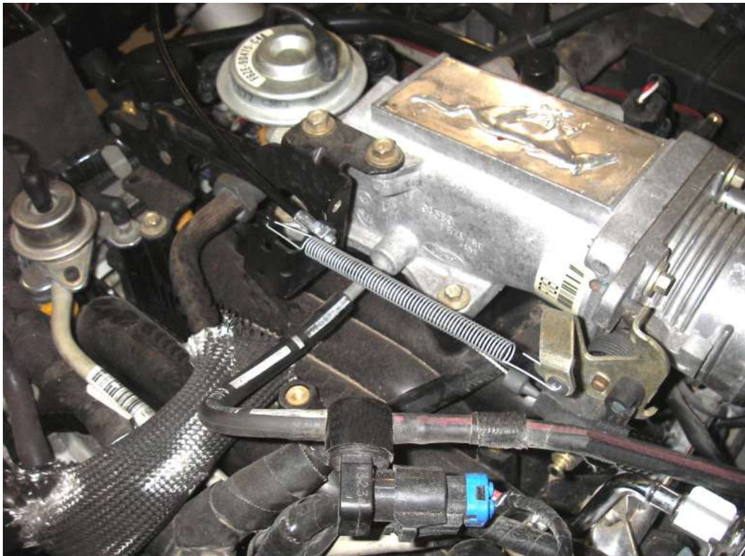
Accelerator cable mounted on 1996 2 valve Intake.
