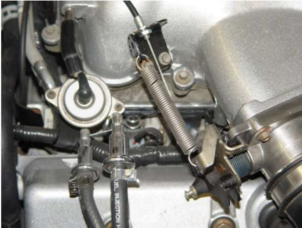
Accelerator cable mounted on 1998 4 valve Intake.
