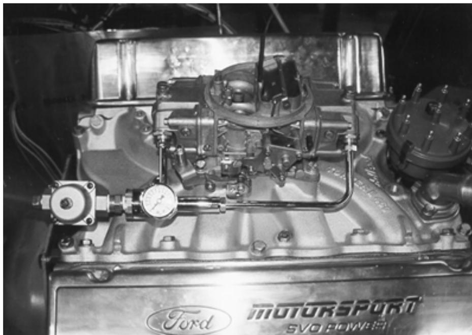
460 Single plane manifold with 850 CFM Carburetor
