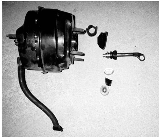
Power booster with the rod removed.
