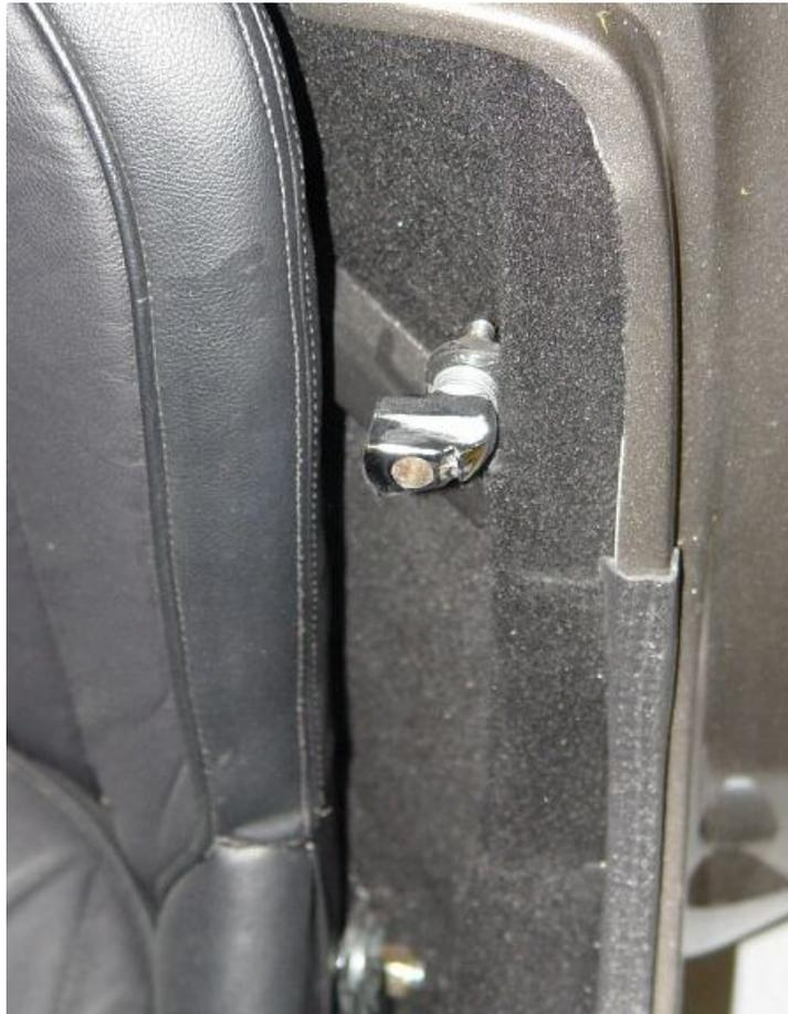
Door striker mounted. Note, seat and carpet are mounted in photo which would not have been done at this time.
