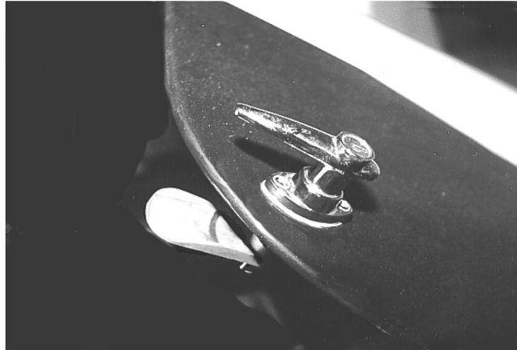
Mounted L-shaped hood handle with cam wedge.
