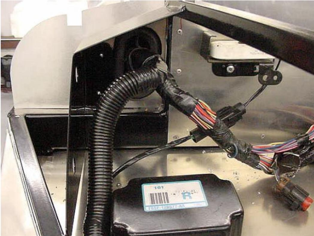
Engine harness passing through firewall extension.
