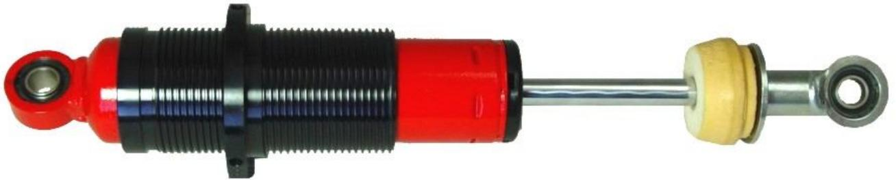
5. The coil-over hats have a snap ring which holds it in place. Remove this snap ring to assemble the coil over shock.
