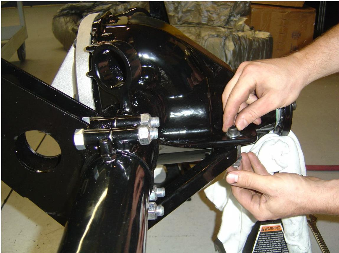
13. Install the rod ends with jam nuts in the upper control arm and bolt the arm in place. One end bolts to the axle bracket just installed and the other end to the bracket welded in at the factory on the passenger side of the 2"x 3" frame rail. Use the spacers and 5/8" bolts provided. The lower bolt hole provides more traction than the upper hole.
