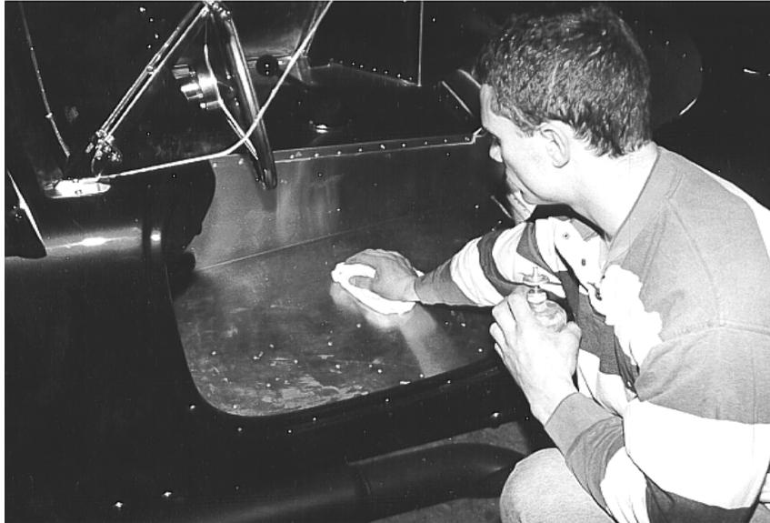
Clean the aluminum cockpit floor before final assembly.
