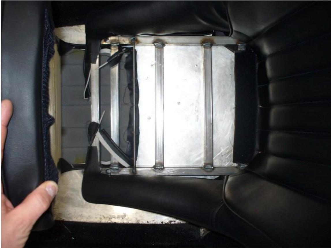
7. If the seat can not get mounted in four places, reposition the seat.
