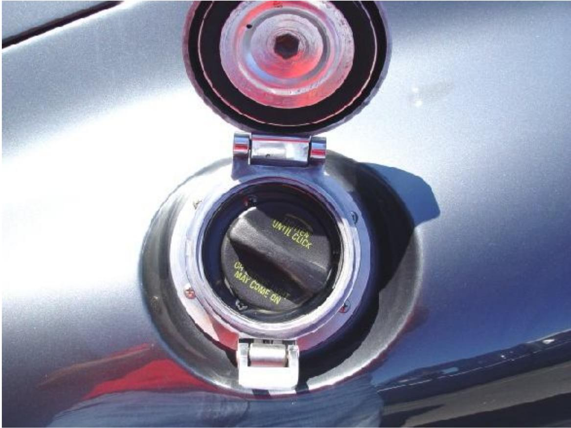
Gas cap located to open towards the center of the body. Note the 1/4 turn gas cap.
