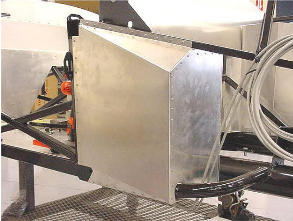
Fuel line routing in front of the passenger foot box.
