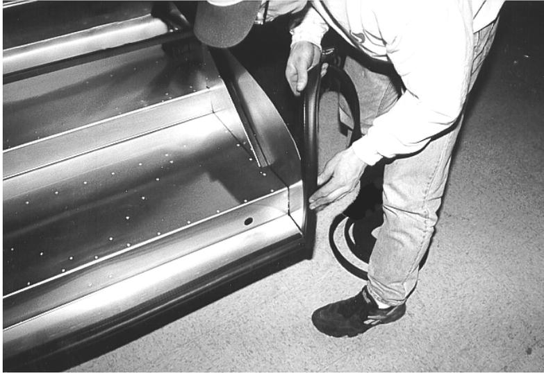
Press on bulb seal on trunk sidewall.
