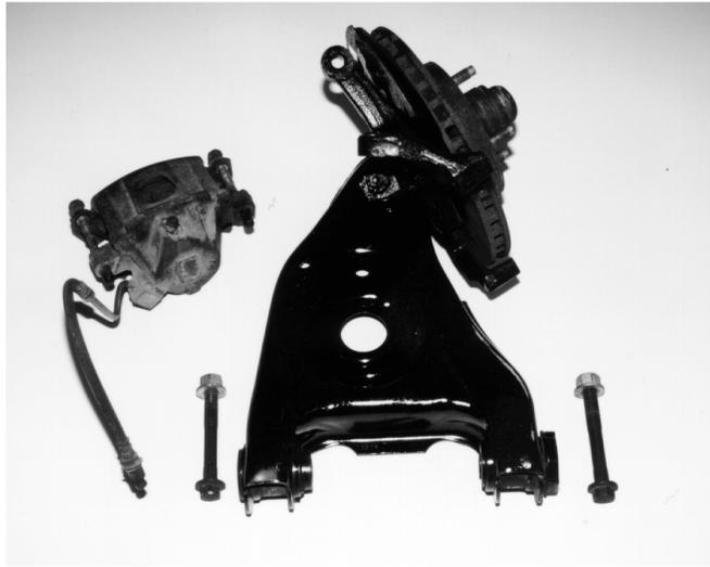
Lower A-arm w/bolts, brake caliper, spindle and brake rotor.
