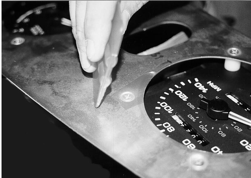
15. Cover each gauge face with paper so that spray adhesive does not get on the gauge faces.
