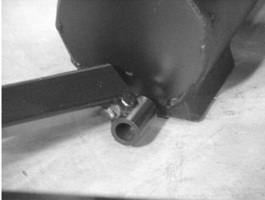
Drill through mount into back of frame
