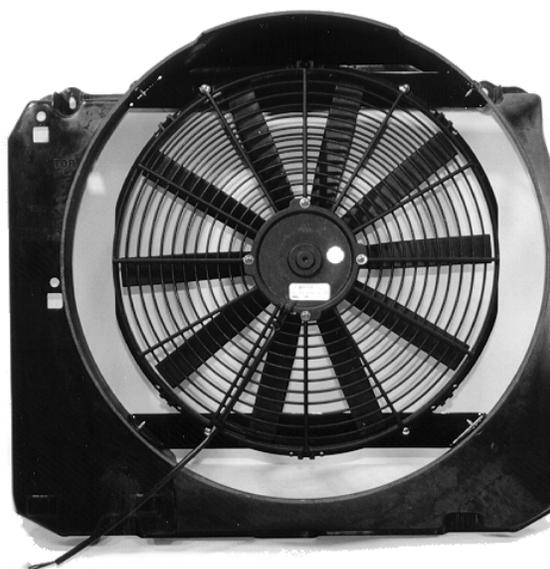
Mustang fan shroud with kit fan and mount strips
