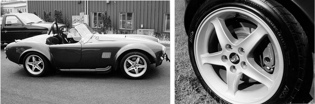
Left: FFR car using late model 17" Cobra-R rims. Right: Ford Motorsport Cobra R 17" wheels and 12" Cobra Brakes.
