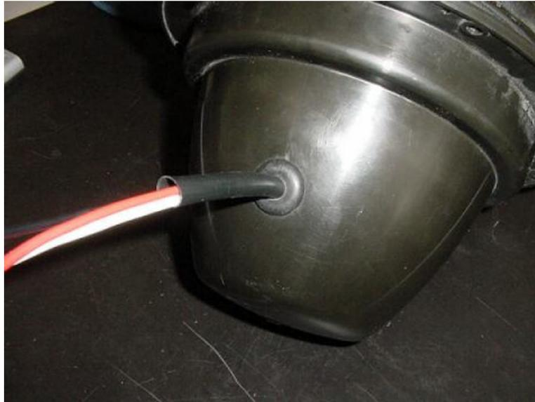
Pigtail wires and covering pulled through grommet.
