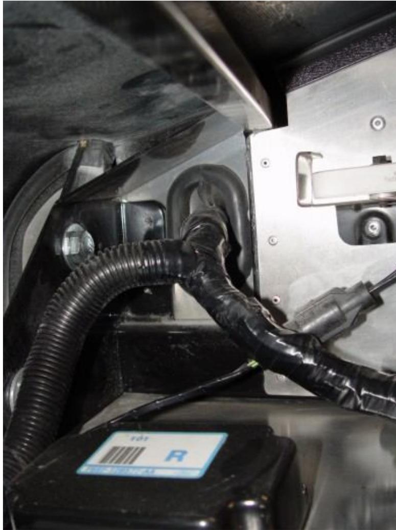
Engine harness plug mounted in firewall.
