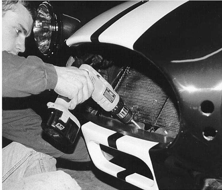
Drilling the radiator and aluminum nose panels.
