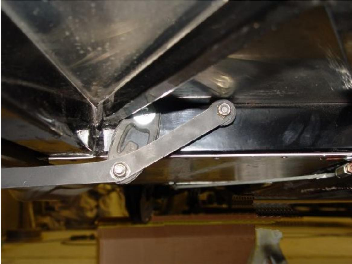
Side Exhaust mount attached to frame.
