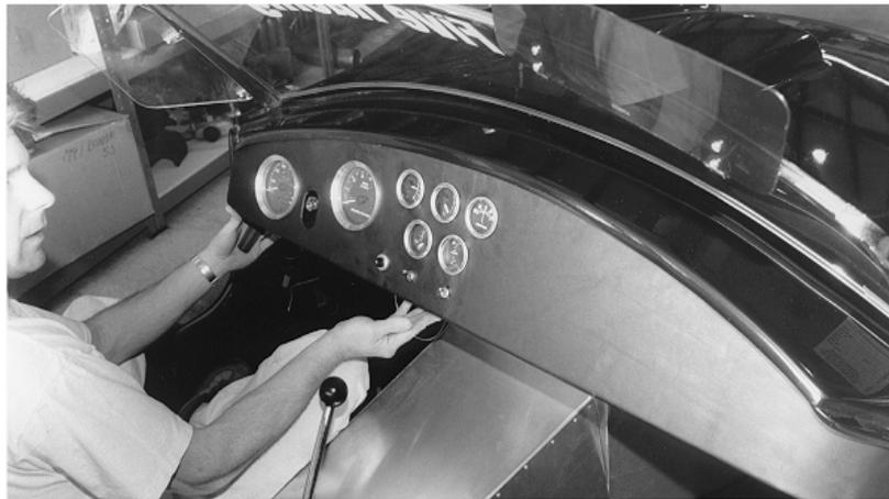
Installation of the dash with Mustang gauge conversion set.
