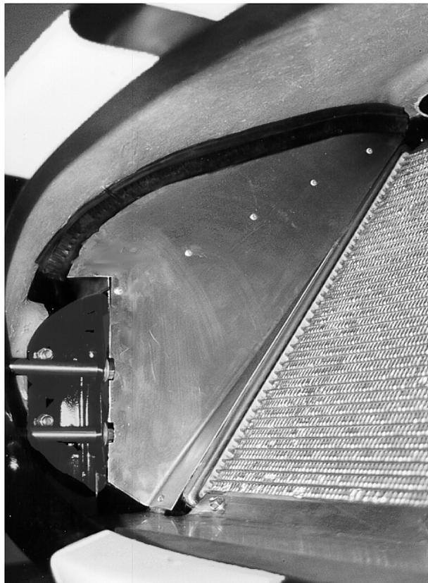
Passenger Side aluminum mounted with weather-stripping.
