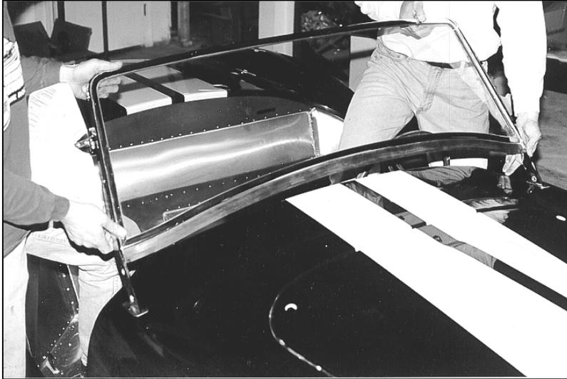
Inserting the windshield into the body.
