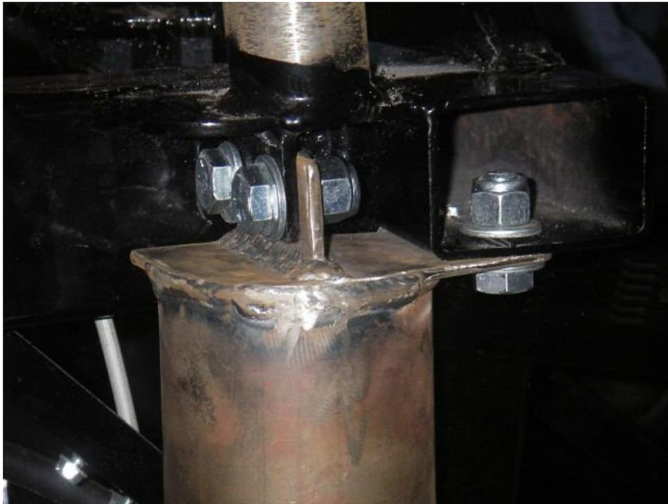
Spring perch mount bolted on frame.
