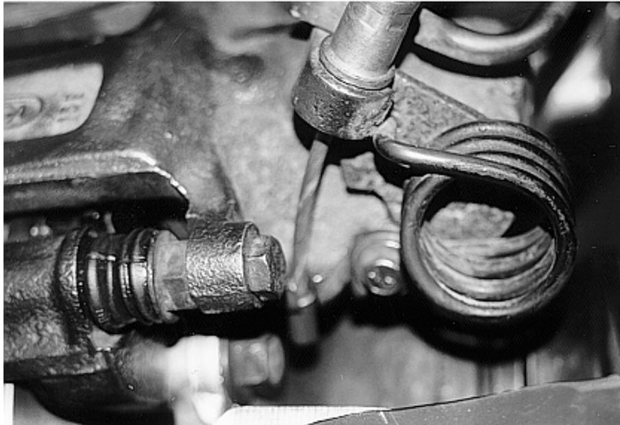
Emergency brake cable in caliper bracket.
